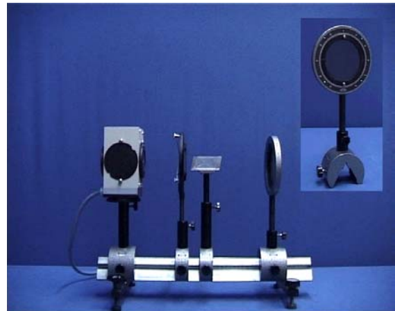
Fig. 2: Setup (f.l.t.r.: Hg-spectral-lamp, aperture plate, calcite-crystal, analyser)
